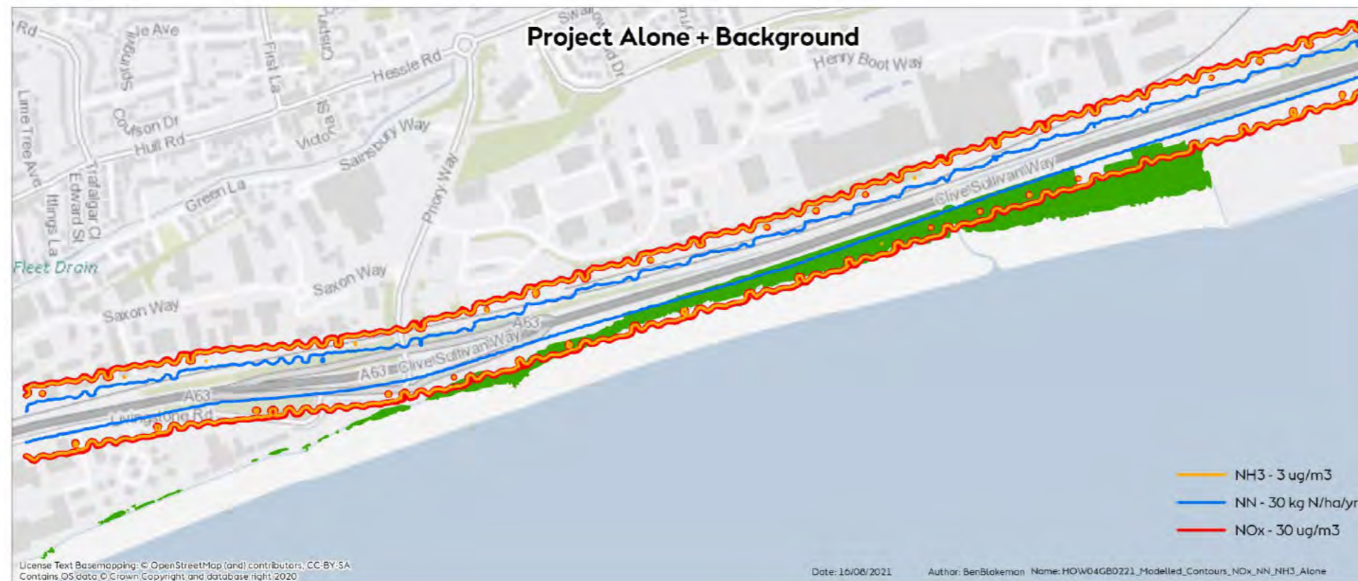
Figure 4: Modelled contours for project contributions (alone where the 1% of critical level/load are reached and with background where the critical load/level is reached) for NOx, NH3 and NN.
